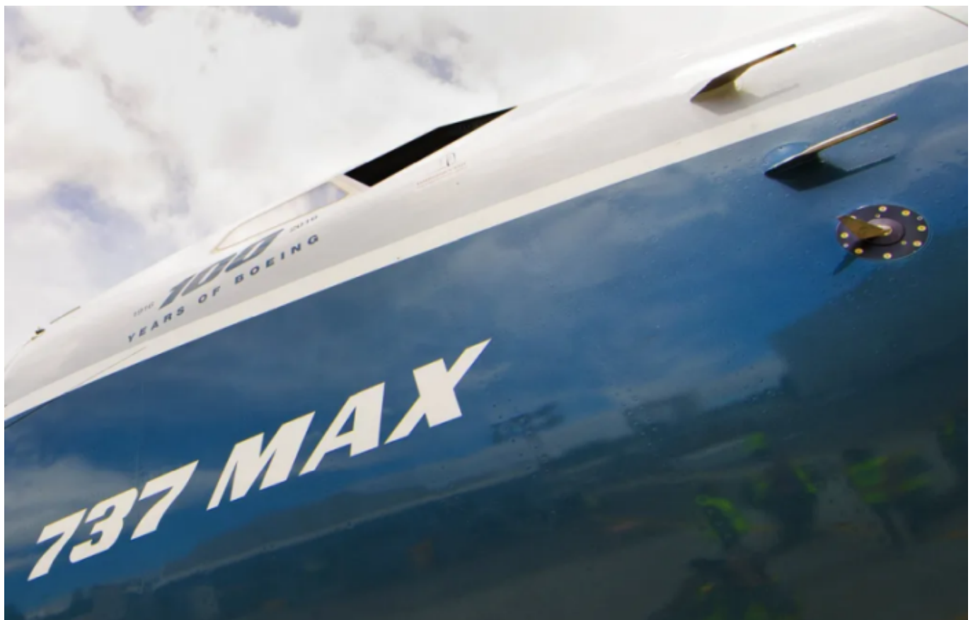
An angle-of-attack sensor is visible on the far right, near the nose of a 737 MAX at Boeing Field in Seattle. Photo: Mike Siegel
